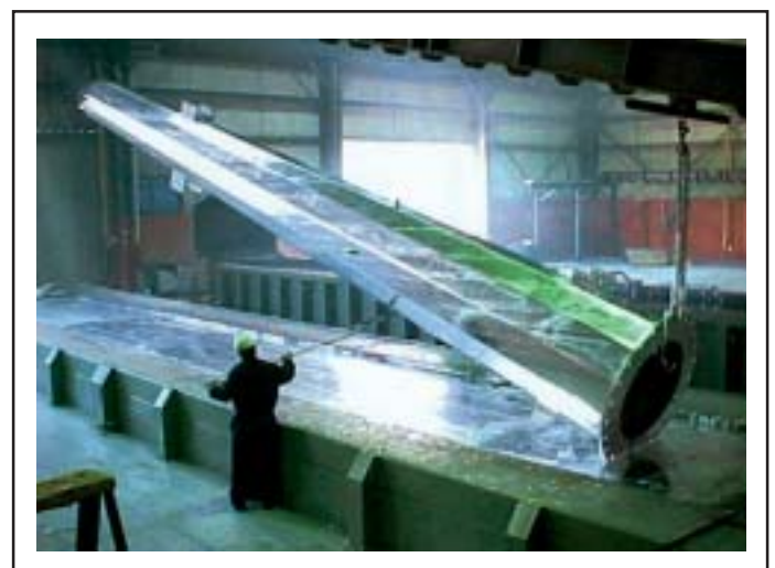
Larger hot dip galvanizing baths allow large structural fabrications such as this power pole to be coated quickly and cost effectively.
